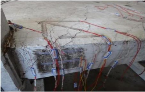
(a) Experimental Cracks of Beam (B) [20]
