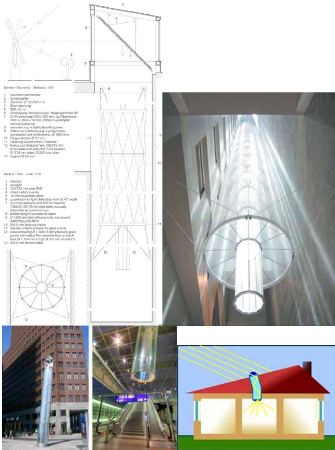
(Fig.10) light tube section design
