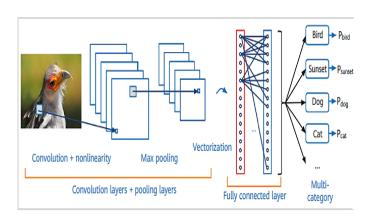
Fig.1 Construction of the CNN deep learning model.
