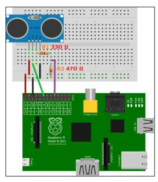
Fig. 5: Schematic diagram of Ultrasonic sensor with Raspberry pi 3.
