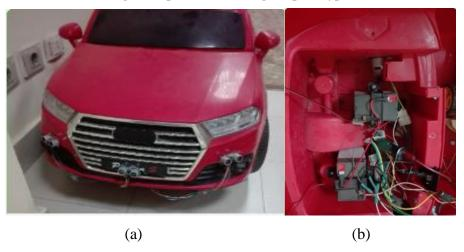
Fig. 4: Parts of hardware components inside the self-driving car prototype (a) front ultrasonic sensors, (b) Batteries and Raspberry pi 3 module.
