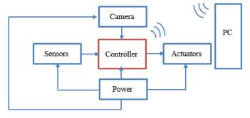
Fig. 2 Generic block diagram of the self-driving car prototype
