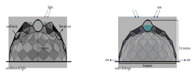
Figure (6) the structure of the tent shows, its dimensions and the design produced for energy
