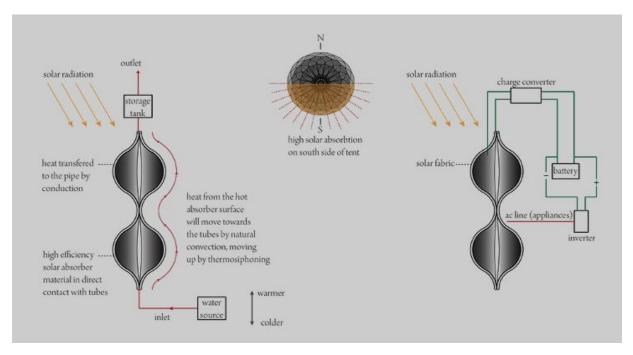
Figure (9) shows the mechanism of water storage and heating and conversion into electrical energy within a battery
