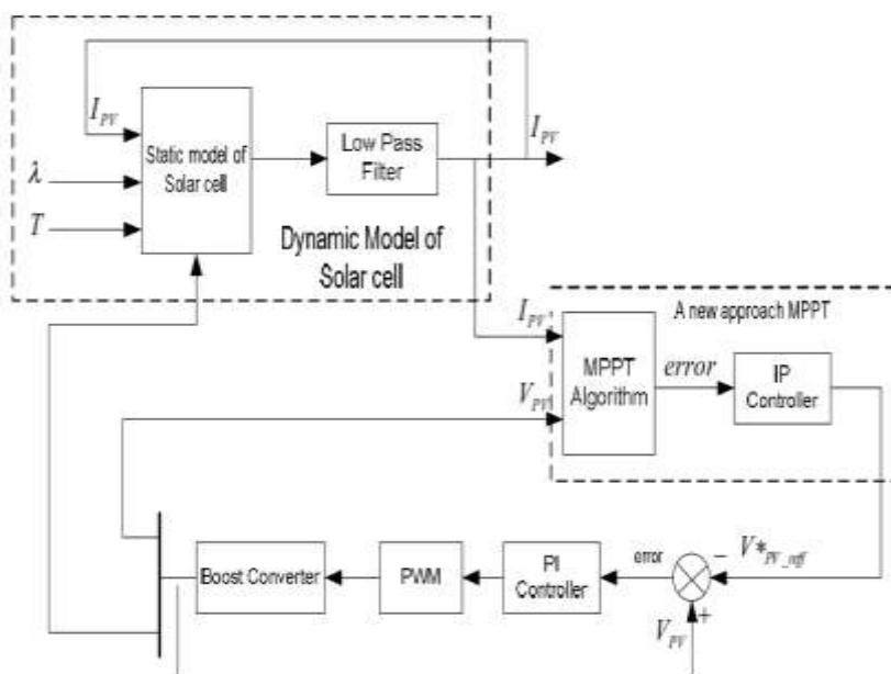
Fig 2 Block diagram of a new MPPT
