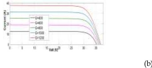
Fig 1.(a) P-V , (b) I-V curves at 25 °C characteristics of solar cell under different irradiance
