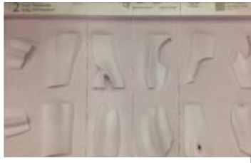
Fig. 42. Molds made of EPS, 2" thick
